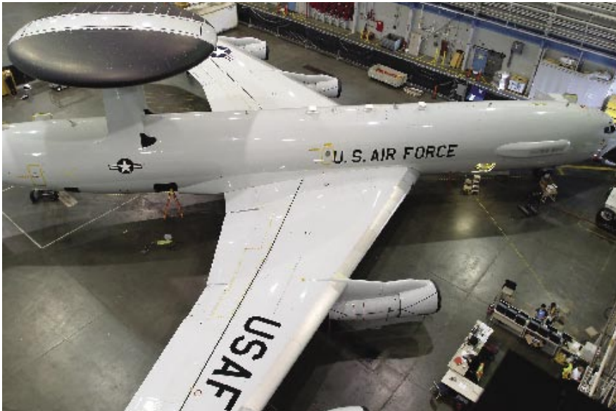
Work begins on the first of 32 E-3 AWACS that will receive a suite of new air traffic management systems and satellite communications. The upgrade, to be finished in 2010, will allow AWACS to fly the most advantageous routes around the world.
