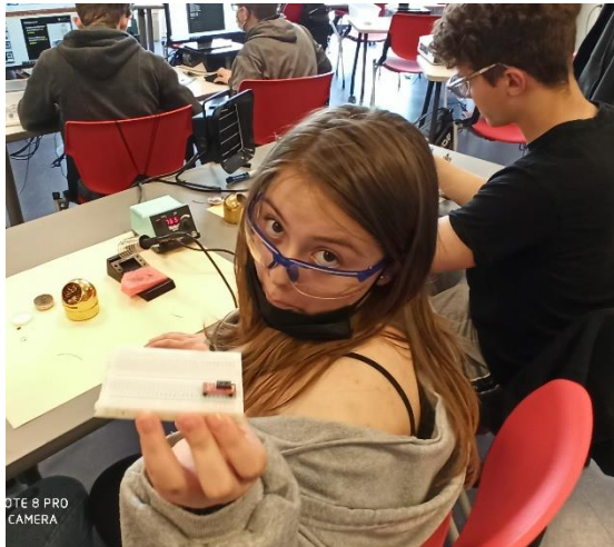
Flight computer build with solderless board containing a humidity sensor -- - and flight computer completed with 3-D printed cases
