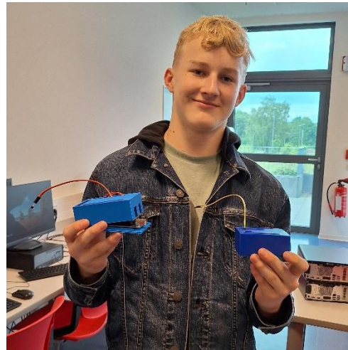
Flight computer build with solderless board containing a humidity sensor -- - and flight computer completed with 3-D printed cases
